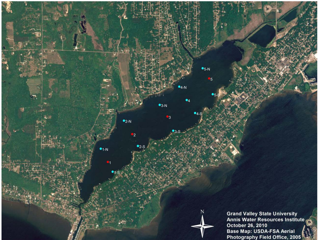
Figure 1. Sampling locations in Bear Lake. Sites 1, 2, 3, and 5 (red dots) were primary coring locations sampled for empirical determination of internal phosphorous loading. All locations (n=15) were sampled for sediment phosphorus, which was used to model estimates of internal phosphorus loading.
