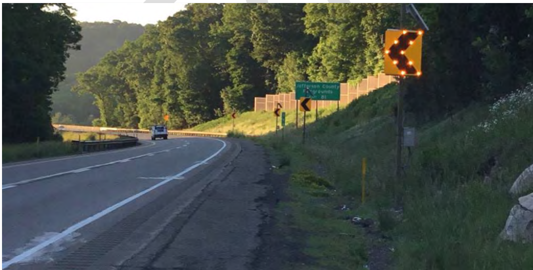
Figure 27 - LED Chevron Sign (PennDOT)
