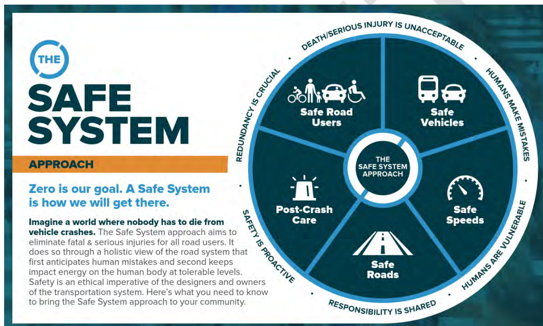
Figure 2 - The Safe System Approach (Source: FHWA)
