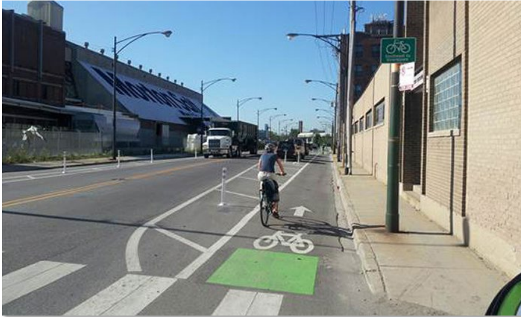
Figure 46 - Buffered Bike Lane (FHWA)
